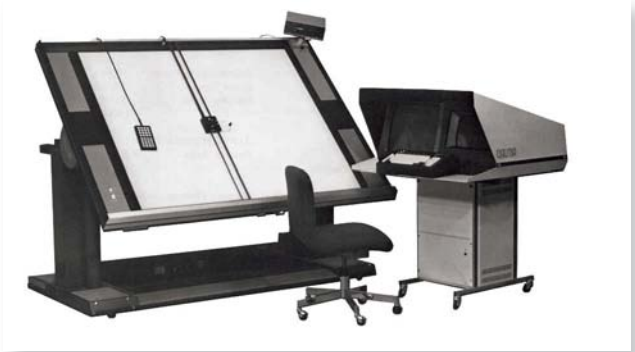
The Calma Digitizer workstation, introduced in 1965, allowed coordinate data to be entered and turned into computer-readable data.
