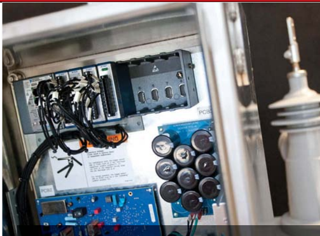
Fig. 3: Smart grid switches and reclosures aim to make the electrical grid as robust and self-healing as the Internet. To achieve this, they must automatically detect problems, isolate faults and redirect power. An NI CompactRIO embedded system (left), the “brain” of the switch, provides a field reconfigurable platform for smart grid R&D by performing multiple measurement, signal processing and control processes in parallel and in real-time. On the right is the output of a CompactRIO-based transformer monitoring system.
